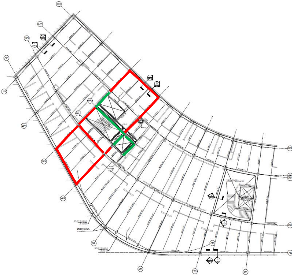
Figure 11: Lateral system in western wing
