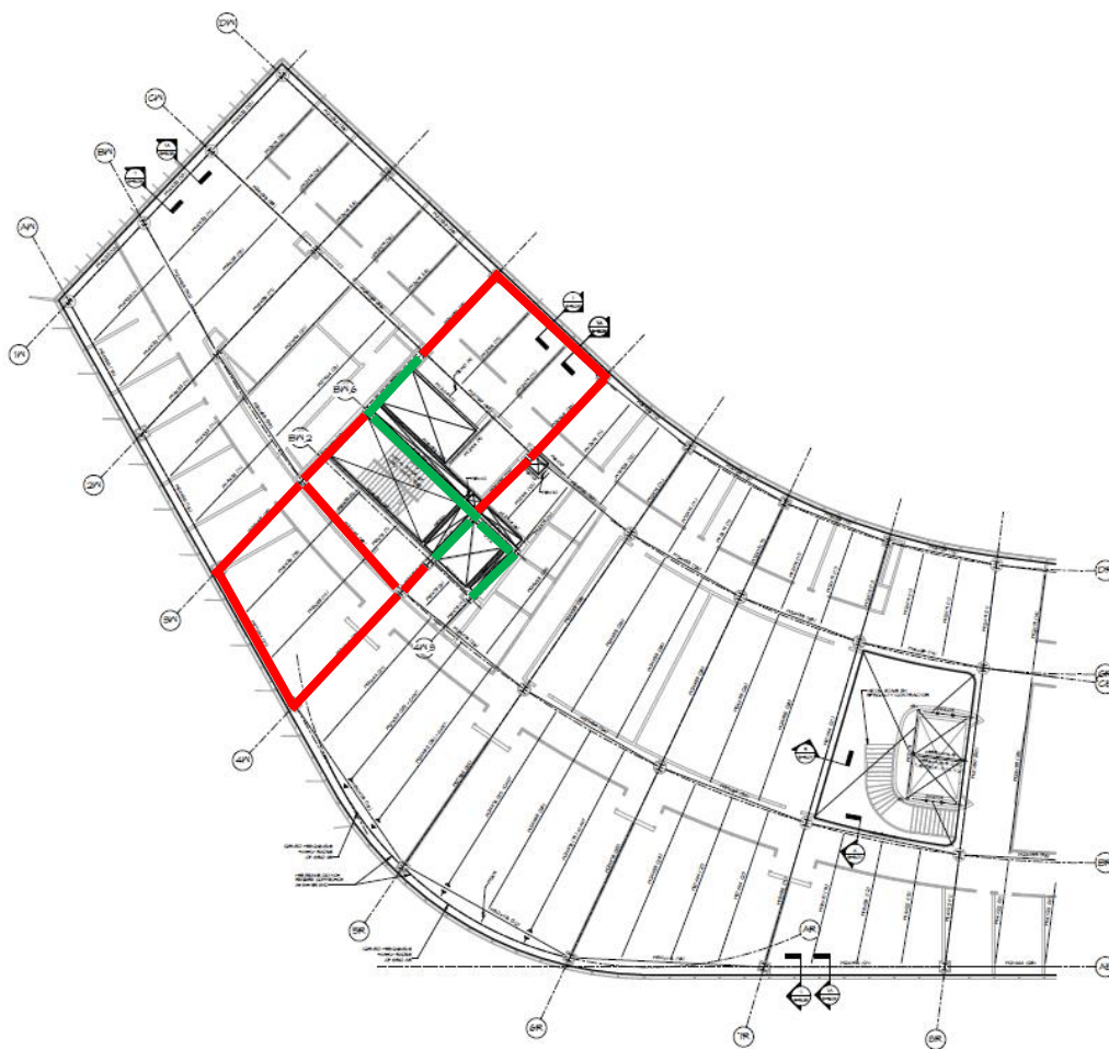
Figure 12: Lateral system in western wing
